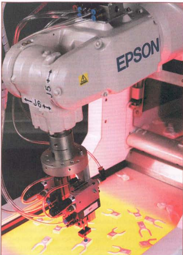
A six-axis robot with vision guidance works with a flexible parts feeder. The parts being processed are for an oral healthcare product. (Photo courtesy Epson Robots)
