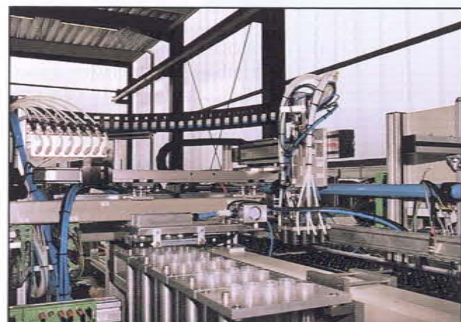
In this assembly application, one-, two- and three-axis solutions combine linear motion systems with motors, cables, and servo drives, as well as interfaces to all commonly used fieldbus systems. (Photo courtesy Bosch Rexroth Corp.)
