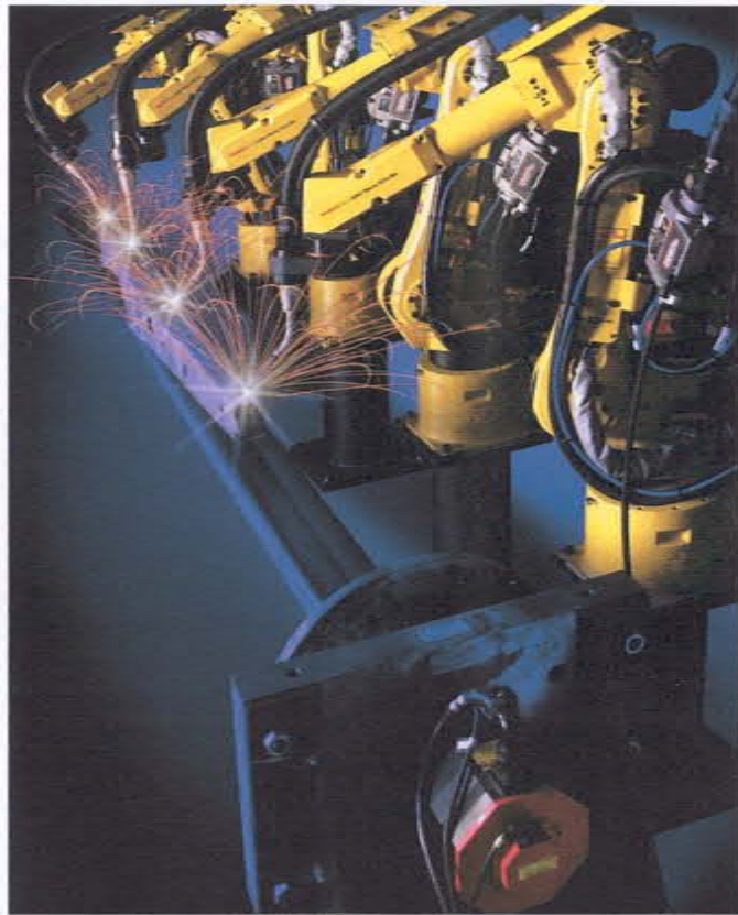
Four robots in this arc welding system work in coordinated motion from one controller. (Photo courtesy Fanuc Robotics)
