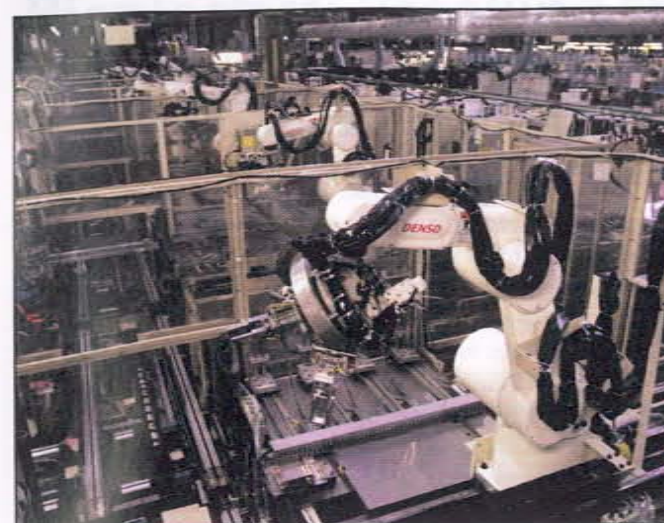
Six-axis robots with multihead end-of-arm tooling (EOAT) assemble automotive parts. (Photo courtesy Denso Robotics)
